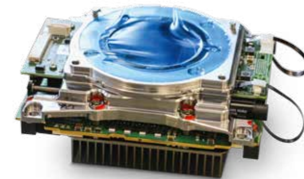
The AMIRA sensor assembly with ND filter slider. One of the two RE 8 motors can be seen at the bottom right.
