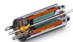
maxon RE 8 motor This drive delivers 0.5 watt of power, at a diameter of only 8 millimeters. It is equipped with precious metal brushes and the ironless maxon winding.
