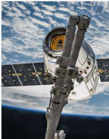
The Dragon capsule developed by Space X, which supplies the ISS with material, uses maxon brushless motors to set the solar sails.
