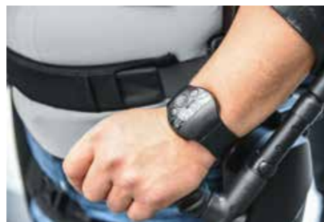
Andre van Rüschen sets his exoskeleton in motion with his wrist-watch-like control device.
